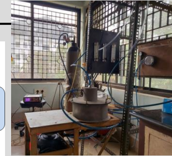
Rotating packed bed for CO 2 capture
