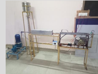
High pressure hydrothermal thermal liquefaction (HTL) reactor for biofuel production
