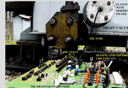
A cost-effective, capacitance-based ppm sensor for transformers
