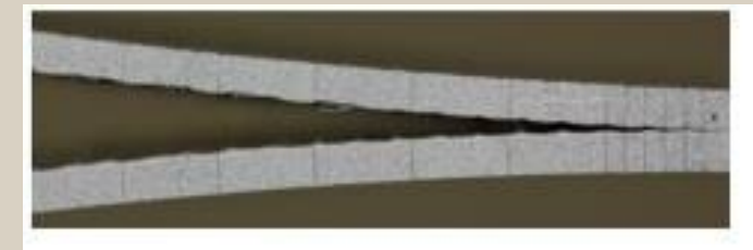
Edge view of bonded joints DCB
