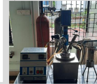
High pressure hydrothermal thermal liquefaction (HTL) reactor for biofuel production
