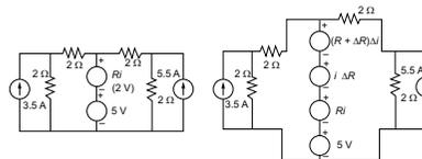
Fig. 5.4-2 Circuits After Applying Substitution Theorem
