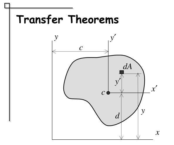
In the above figure, x' and y' are the centroidal axis.
