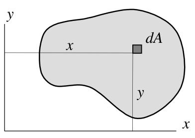
The first moment of a coplanar surface of area *A* about the *x*-axis is defined as
