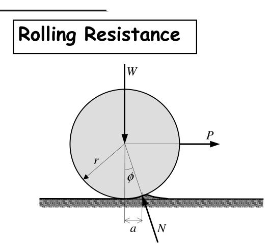
Consider a hard roller, supporting a load *W* at the centre, moving without slipping along a horizontal surface.
