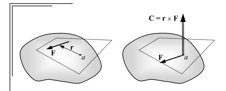
Example: Move the force to the tip and obtain an equivalent force system.
