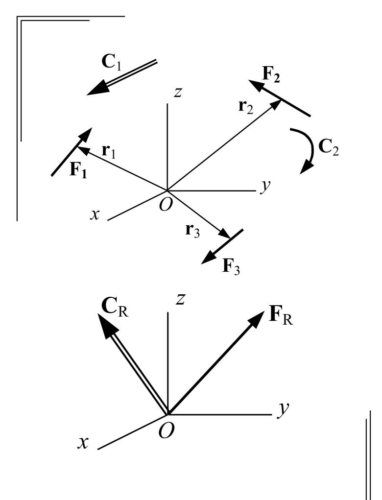
Thus, any force system can be replaced by equivalents no more complex than a single force and a single couple moment.
