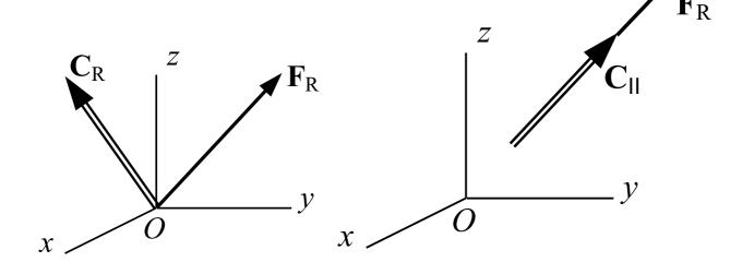
We can resolve  $C_R$  into two components  $C_{II}$  and  $C_{\perp}$ , collinear and perpendicular to the force  $F_R$ .
