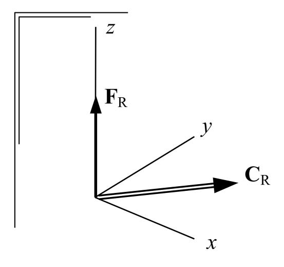
If  $F_R \neq 0$ , we have  $C_R$  lying parallel to xy plane; we can eliminate  $C_R$  by moving  $F_R$  to a new location  $(\bar{x}, \bar{y})$
