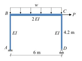
2. The frame shown in Fig. 2 is loaded as shown. Determine all the support reactions and draw the bending moment diagram. E = 200 GPa,  $I = (3.8 + 0.1 \times S) \times 10^{-4} \text{ m}^4$ ,  $w = 6.3 + 0.2 \times S \text{ kN/m}$ ,  $P = 22 + 0.4 \times S \text{ kN}$ . Determine the vertical deflection of point *B*.
